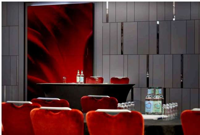
Wall Cladding HPL Cladding Polished Stainless Steel Inserts Digital Printed Glass Artwork
