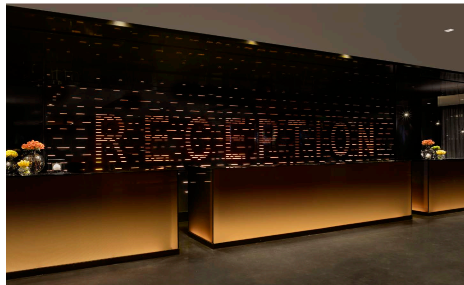
Park Plaza Waterloo - London Digital Printed Glass Front with Edge Lighting DuPont™ Corian® Top Steel Interior Structure Powder Coated Metal
