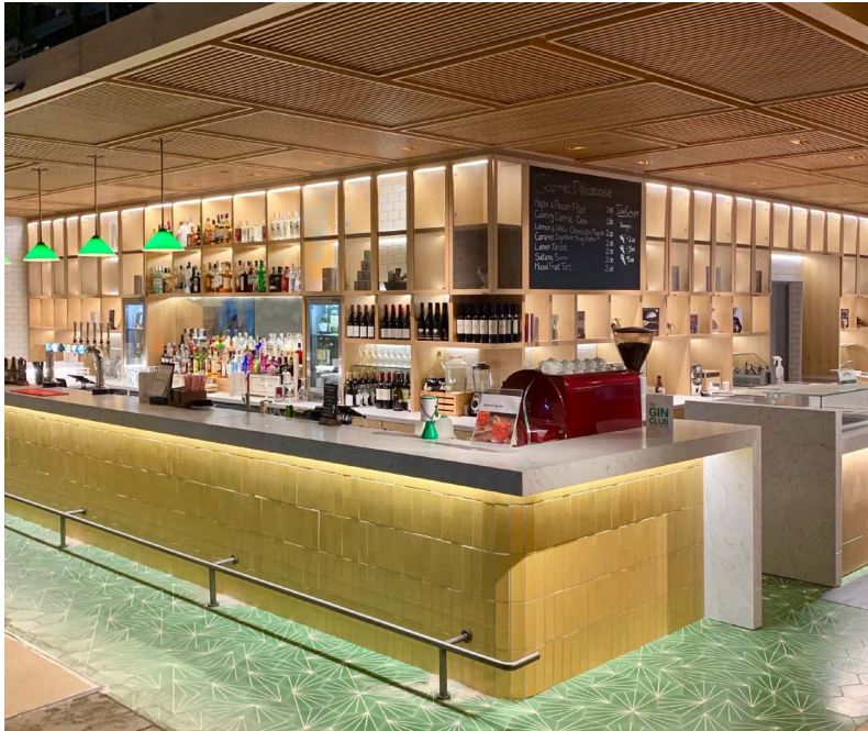
Bar Oak Veneered MDF Slatted Ceiling Marble Top and Integrated Lighting Oak Veneered Cabinets with Metal Mesh Doors
