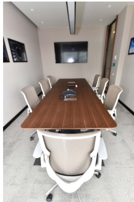
Meeting Table Veneered MDF Top with Varnish Powder Coated Metal Leg
