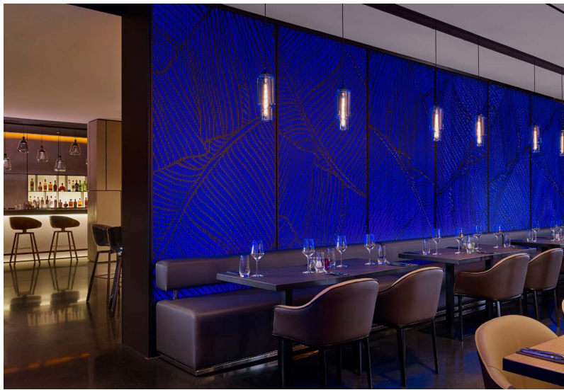
Park Plaza Park Royal - London Laminated Tempered Glass with Digital Printed PVB Powder Coated Metal Frame
