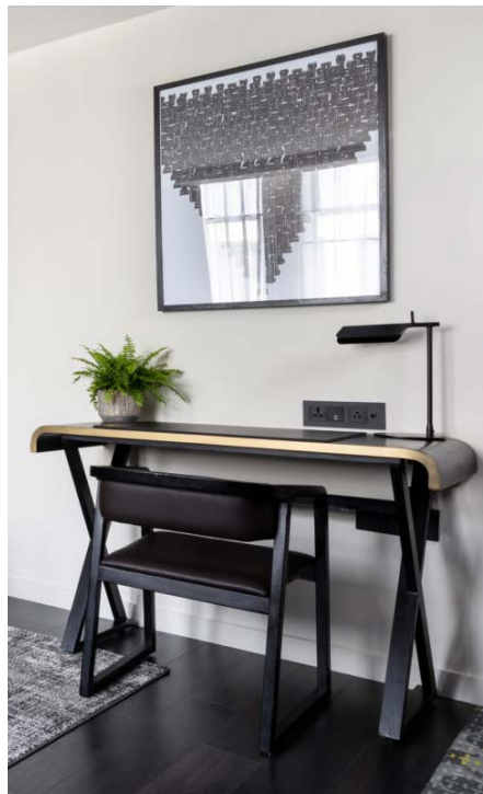
Desk Black Painted Veneered MDF Top Brass Plated Metal Trims Solid Wooden Legs
