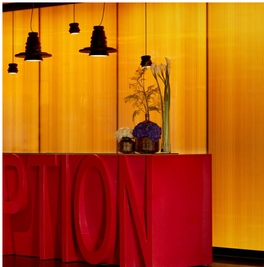
Park Plaza Park Royal - London Laminated Tempered Glass with Coloured EVA Backlighting Powder Coated Metal Skirting
